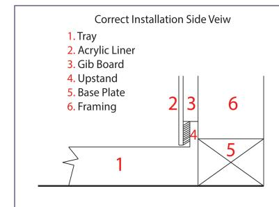
Pictured Left, is a drawing depicting the correct installtion method of a tray in a standard GIB Board Lined Wall.
